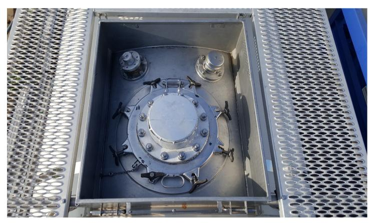
Hydrogen Peroxide tank requirements fall under 49 CFR 173.225 Packaging requirements and other provisions for organic peroxides. Breather vent and bursting disc are required. Top discharge only is required for peroxides over 60% concentration. Proper maintenance and handling is required.
